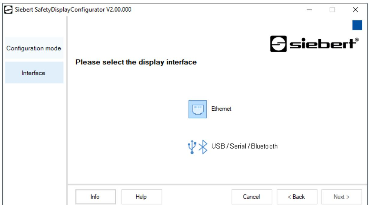
If your display is connected to the PC via a network choose 'Ethernet'.
